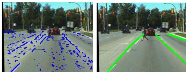
Figure 4.2: a) (left): Lane features detected by Algorithm 1 b) (right): Projected lane splines on the image
