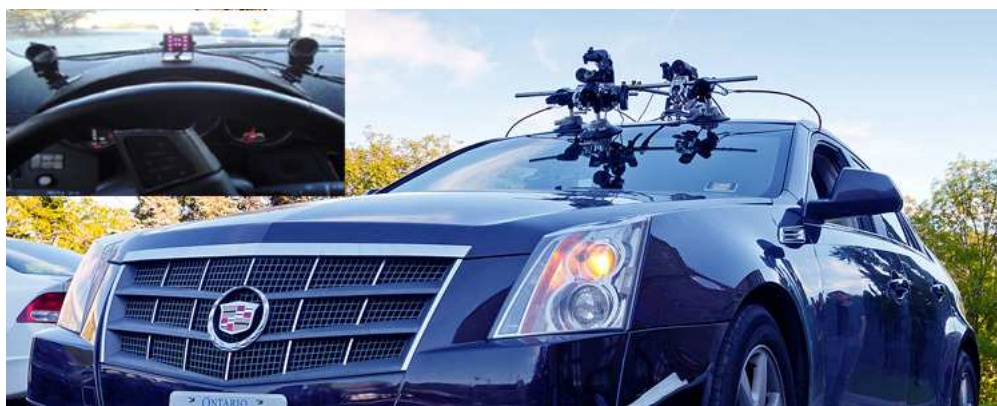
Figure 1.2: Vehicular instrumentation configuration in RoadLAB.
