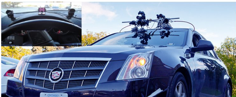
Figure 3.1: Physical configuration of the experimental vehicle with the external stereo cameras mounted on the roof. The dashboard-mounted eye tracker is displayed in the top-left part of the image.
